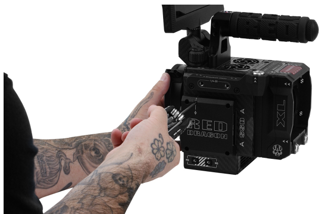
Figure: 取下固定螺丝
