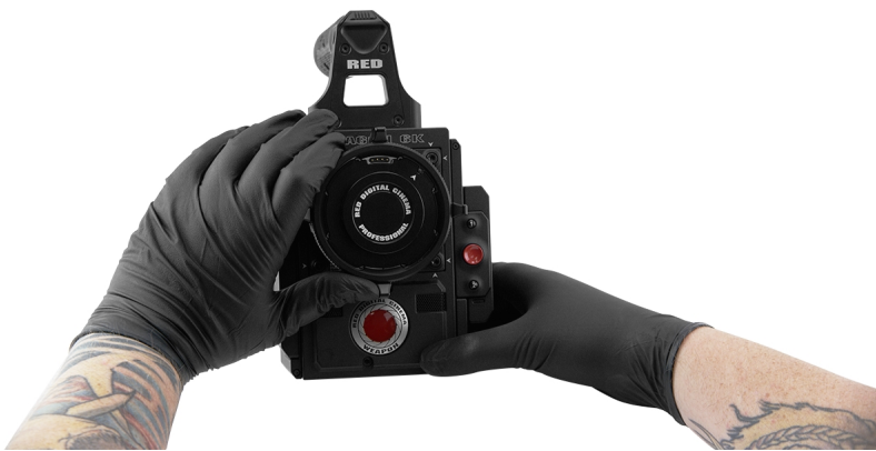
Figure: 顺时针旋转锁定环
