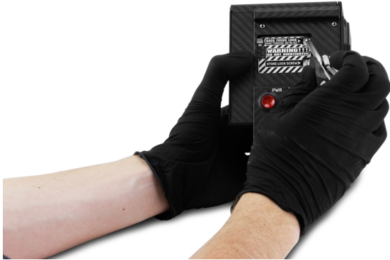
Figure: 锁住后焦点
