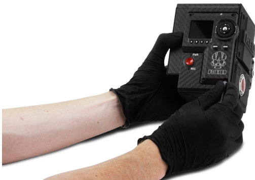
Figure: 卸下 DSMC2 Sidekick
