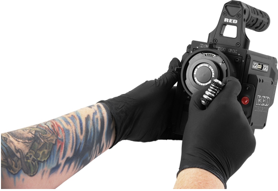
Figure: 拆下镜头卡口螺丝
