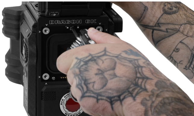
Figure: 逆时针旋转锁
