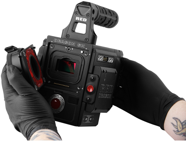
Figure: 拆下镜头卡口
